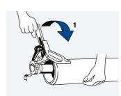
The pipe should be chamfered to approximately 15° and lubricated with suitable Polypipe product. Do not use oil or grease which can damage the rubber seal.
