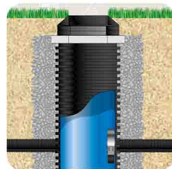
Hydro International Hydrobrake Flow Control Chamber
