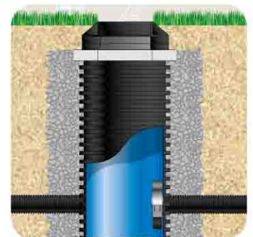
Hydro International Hydrobrake Flow Control Chamber
