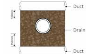
Minimum clearance between duct and drain
