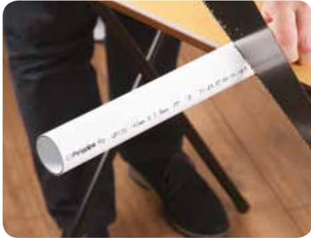
2. Chamfer the end of the pipe to prevent the ring seal being damaged or misplaced when the pipe is inserted into the socket. Fittings with spigot ends are moulded with a chamfer during manufacture.
