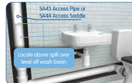
For multi-storey domestic buildings, access into the stack should be provided at 3 storey intervals and for multi-storey commercial buildings access should be provided on each floor.
