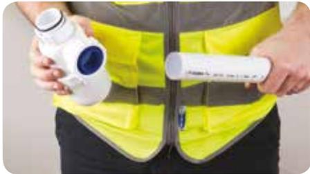
1. Remove the threaded nut, blue finned rubber seal, and blue spacer from the outlet of your trap.
