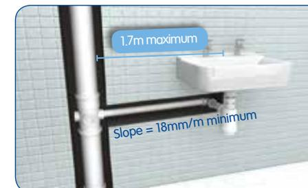
1. Where maximum length is exceeded, an anti-siphon trap or anti-siphon unit should be used.
