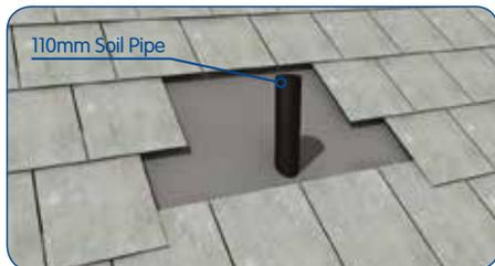
The base plate is dressed to the profile of the lower tiles with the side and upper tiles laid over the top of the base plate. On low pitched roofs, a single welt can be made to the lower edge of the base plate to provide extra strength.
