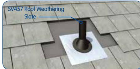
The base plate may be trimmed if required, provided that at least 150mm of weathering remains.
