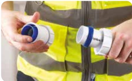
4. Polypipe's blue Fit-Rite™ insertion aid can be left in the body of the fitting if you are connecting to solvent weld and Push-fit pipe. If you are connecting to metal pipe or distorted plastic pipe you can remove the pipe insertion aid.
