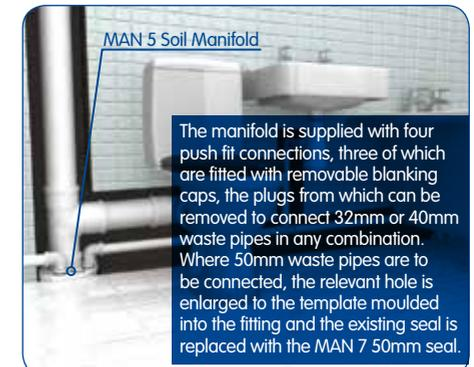
The manifold is supplied with four push fit connections, three of which are fitted with removable blanking caps, the plugs from which can be removed to connect 32mm or 40mm waste pipes in any combination. Where 50mm waste pipes are to be connected, the relevant hole is enlarged to the template moulded into the fitting and the existing seal is replaced with the MAN 7 50mm seal.
