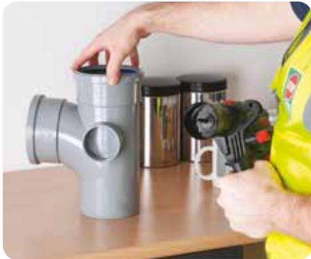
2. Using a drill with a 60mm hole cutter, drill your desired hole.
