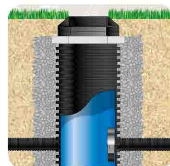
Hydro International Hydrobrake Flow Control Chamber
