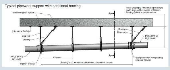
The type of pipe hanger clip or hoop used shall be selected according to the application, special provision being made in instances where the pipework installation is subject to axial movement due to thermal expansion and/or contraction.
