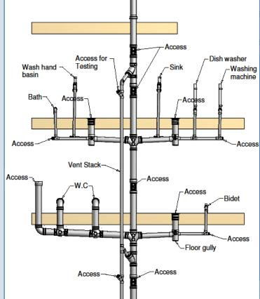
The size of the access point within a building should generally be the same size as the pipework, up to 160mm.
