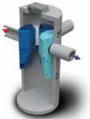
Fig.3a Inlet configurations for all models include options for inlet grates and multiple inlet pipes.
